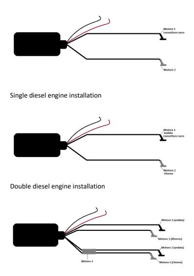
Motore 1: Left engine looking at the bow Motore 2: Right engine looking at the bow
