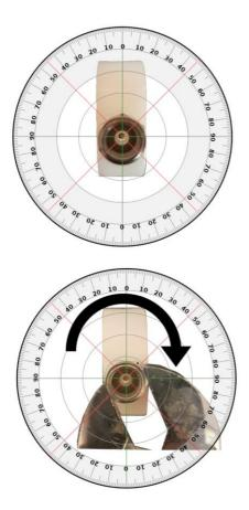
Do not tighten beyond 40 degrees as the thread could break.
